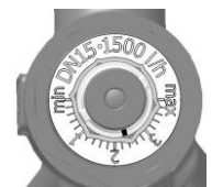
Ring with dial for presetting (B)
