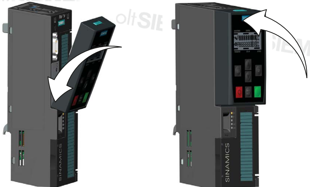
Figure 3-1 Fitting the BOP-2 to the Control Unit
