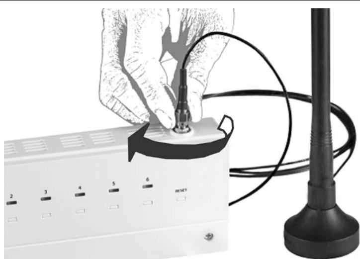
**en** In case of weak connectivity of the RF signal between wireless thermostat (RDD / RDE) and the multizone receiver (or special installation inside a metal enclosure), the user has the option to mount an external antenna.
