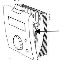
Remove base and open housing by pushing down at the top with a screwdriver.
