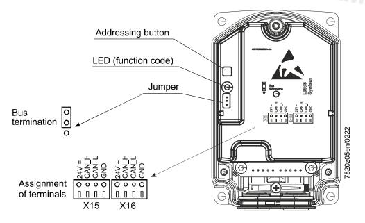
The two connection jacks (X15, X16) are identical.
