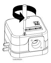
Step 3: Attach the M20 cable gland (the cable gland is not included in the scope of delivery).
