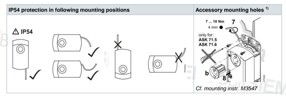
$oldsymbol{\Lambda}$   $^{1)}$ Not to be used for fixation of the actuator, use anti-rotation-bracket instead.
