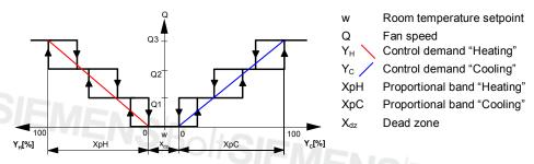
Note: The diagram only shows the PI thermostat's proportional part.
