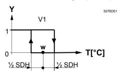
Cooling mode with manual selection (P01=2) or for P09 >= P10 in cooling sequence \*)
