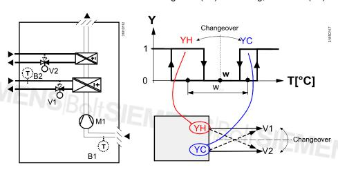
Note: This example shows ON/OFF control; for modulating control, connect the appropriate output terminals
