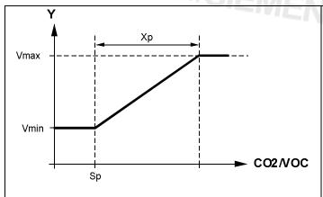
Sp: CO<sub>2</sub> setpoint [P19] Xp: CO<sub>2</sub> proportional band [P20] Vmin: Minimum flow
