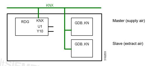
Parallel connection of Y10 control signal and air damper position feedback via U1
