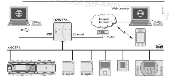
The OZW772 web server enables users to operate a Synco HVAC system from a remote location – via PC or from a smartphone via the web. A start page shows the most important data points. A combination of menu/path navigation enables users to access all data points quickly and straightforwardly. The entire installation can be visualized in the form of plant diagrams. Alarm and state messages can be forwarded to different message receivers, such as e-mail, SMS, etc.
