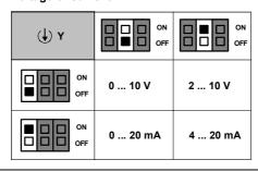
Assignment of correcting span Y and U:
